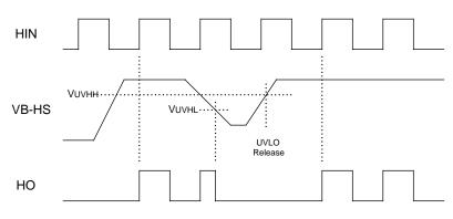
After UVLO is released, IC operation is started by the first rising edge of input
