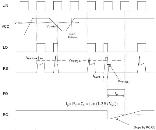
After UVLO is released, IC operation is started by the first rising edge of input
